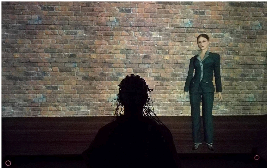
Fig. 2. A participant in the experiment, wearing a 64-channel EEG cap, listening to virtual agent Emily in the CAVE environment. By wearing 3D shutter glasses, participants experienced the projected immersive virtual environments in 3D.
